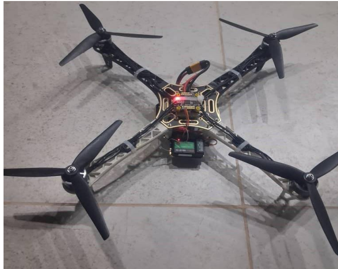
Figure 6. Drone prototype with Speedy Bee F405 V3 Controller, Used for research on Flight stability and real time data processing
