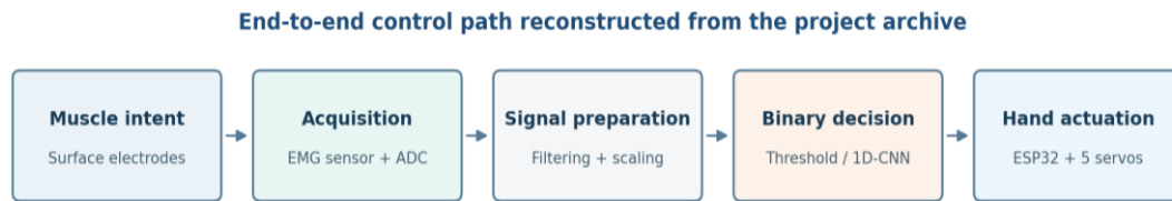
Figure 1. Reconstructed sensing-to-actuation and data path. The compact 1D-CNN is retained as an archived mapping stage; exact on-device CNN inference is not claimed.
