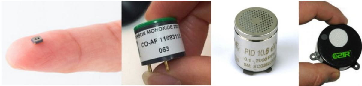
Figure 4. Examples of low-cost chemical sensors. (from left to right) MOX sensor (Model: FigaroTGS 8100); AGS sensor (Model: Alphasense CO-AF); PID (Model: RAE Systems PID 10.6 eV); (d) NDIR sensor (Model: CozIR by Gas Sensing Solutions) [50].
