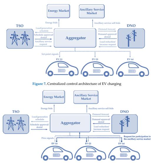
Figure 8. The block diagram of the decentralized control architecture.
