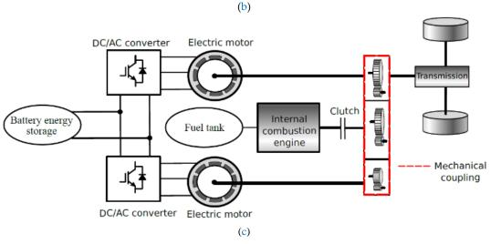
**Figure 4**. The diagram of full hybrid EV classification. (a) Series hybrid EV, (b) Parallel hybrid EV, (c) Parallel–series hybrid EV.
