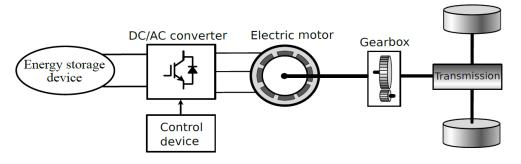
Figure 2. The diagram of battery electric vehicles.
