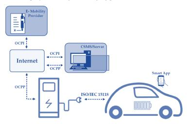
Figure 9. The communication protocols utilized during the charging procedure.
