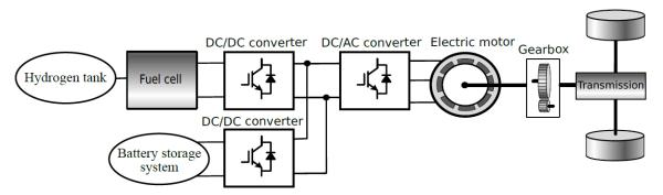
Figure 3. The diagram of fuel cell electric vehicles
