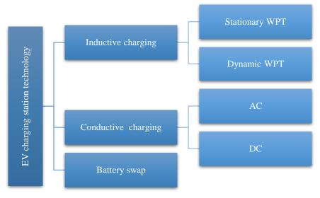
Figure 5. Three primary types of EV charging technologies
